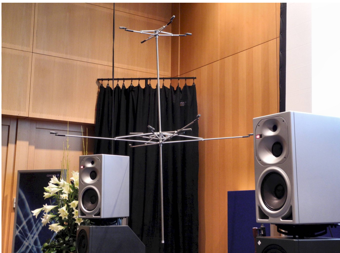
FIGURE 8 – THE 12 CHANNEL 3D MULTIFORMAT MICROPHONE ARRAY SUPPORT SYSTEM CALLED THE ‘WILLIAMS 12 CHANNEL UMBRELLA’ (PHOTO BY KIND PERMISSION OF JORG WUTTKE TAKEN AT THE 2012 TONMEISTERTAGUNG IN KÖLN)
